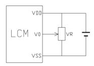
VDD~V0: LCD Driving voltage
